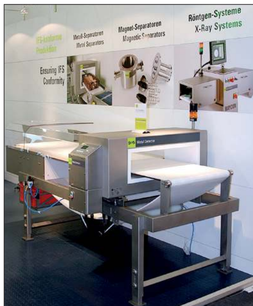
UNICON metal detection system with retracting belt
