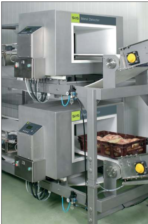
Metal inspection of poultry in E1 containers
