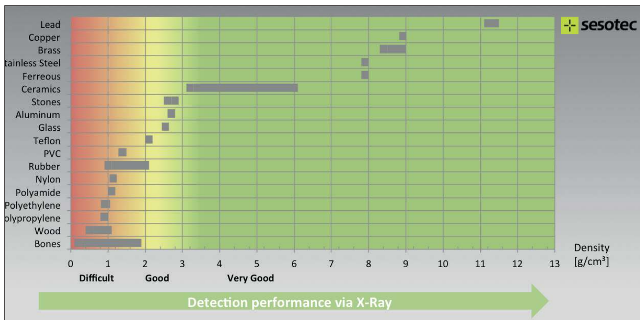
Detection capability for different materials categorized by density.
