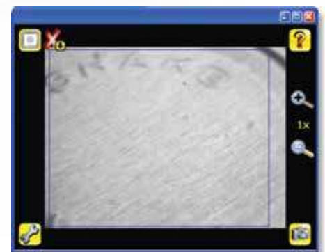
Can end missing date code
